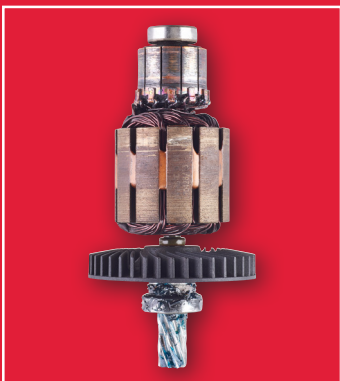
Burnt motor due to overload
