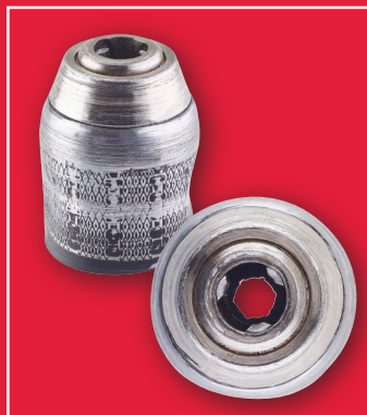
Broken chuck due to misuse
