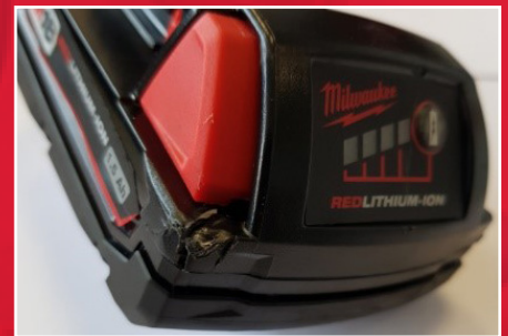
Example of an external force (heavy impact)
