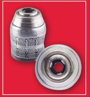
Broken chuck due to misuse
