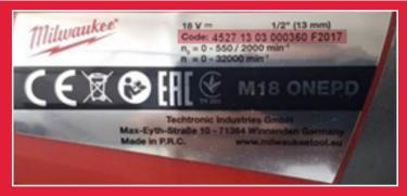
Production codes are located on the rating label outside of the unit. The production code on the tool (shown above) should match the Warranty certificate (shown to the left).
