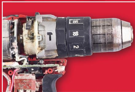
Example of excessive wear and tear
