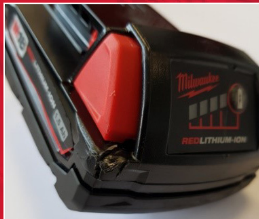
Example of an extreme drop or impact of a MILWAUKEE® battery
