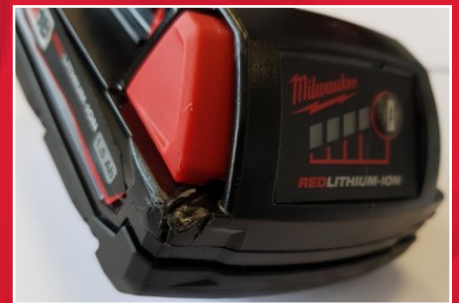
Example of an external force (heavy impact)
