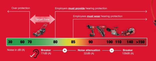
SNR (Single Number Rating) = attenuation in dB H/M/L = High-/ Medium- /Low-frequency attenuation value
